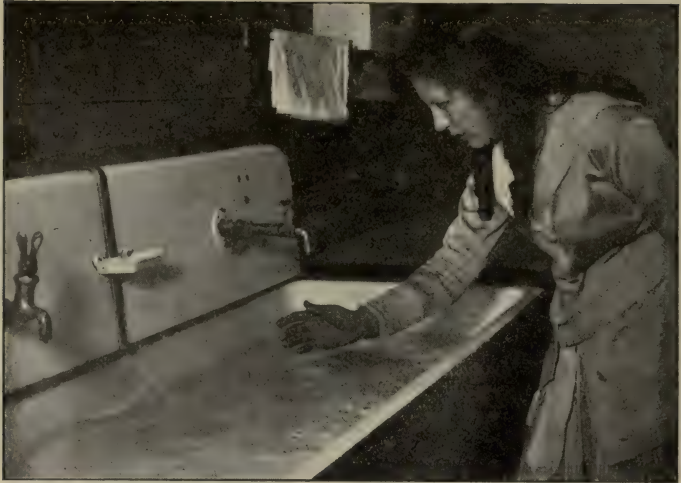
FIG. 102. When the wave reaches the end of the sink, it is reflected back. Sound waves are reflected in the same way.
